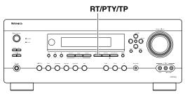
When tuned to an RDS station that's broadcasting text information, the text can be displayed.
